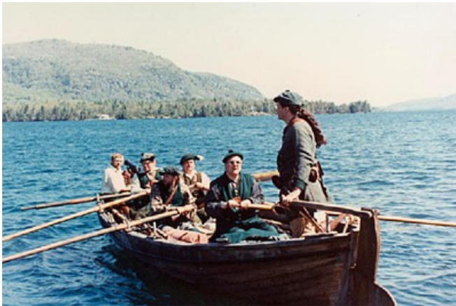
A good perspective of single bank rowing, note the lapstrake construction. We are approaching Sabbath Day point
