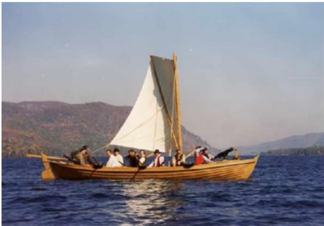
The whaleboat in it's final full form. Based on Rogers Expedition to Detroit, we added a small sprit sail rig.
